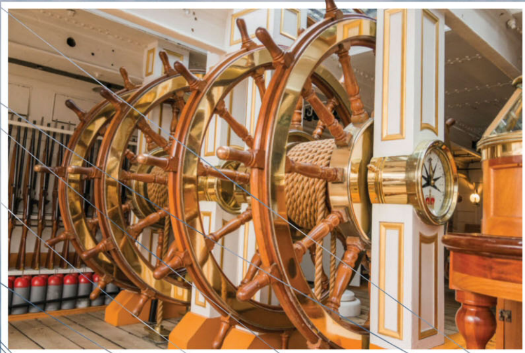
Above: Warrior had three sets of wheels on different decks. These wheels are on the gun deck and are known as 'battle wheels' as they were for use in action. It took eight men to operate them
